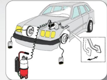
*Air-operated brake-bleeder tank for brake and clutch bleeding also with ABS.*
